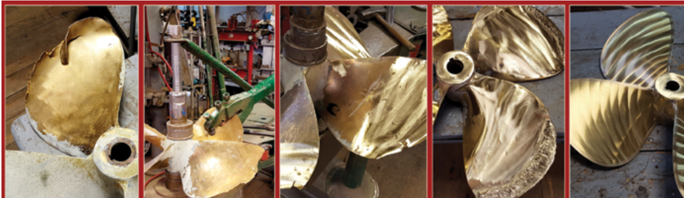
When a commercial boat's propeller literally hits rock bottom, it goes to Union for reconstruction processes that only a few marine machinists know: bending blades back into alignment with heat and a 6-foot lever; grinding down to good metal; building up with welds; and last, grinding, balancing and applying Union's signature finish.
